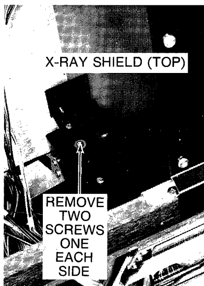
Fig. 16a — Upper X-Ray Shield
